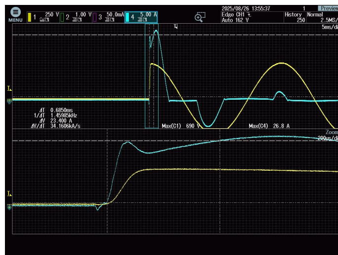
Figure 1. Inrush Current @ full load and cold start
