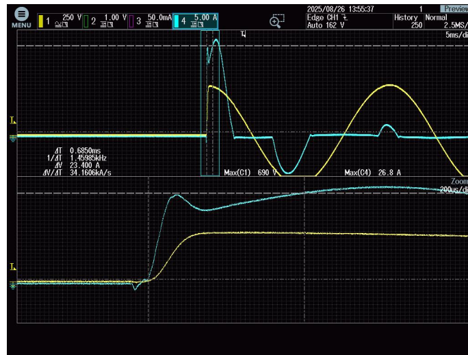
Figure 1. Inrush Current @ full load and cold start
